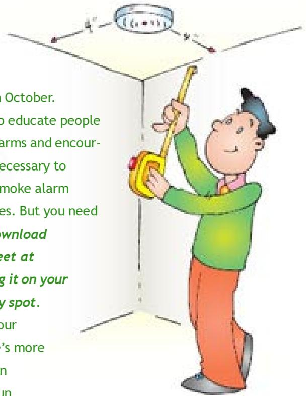
Smoke rises; install smoke alarms following manufacturer's instructions high on a wall or on a ceiling. Save manufacturer's instructions for testing and maintenance.
